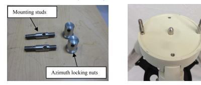
Figure 13. Mounting studs and locking nuts
